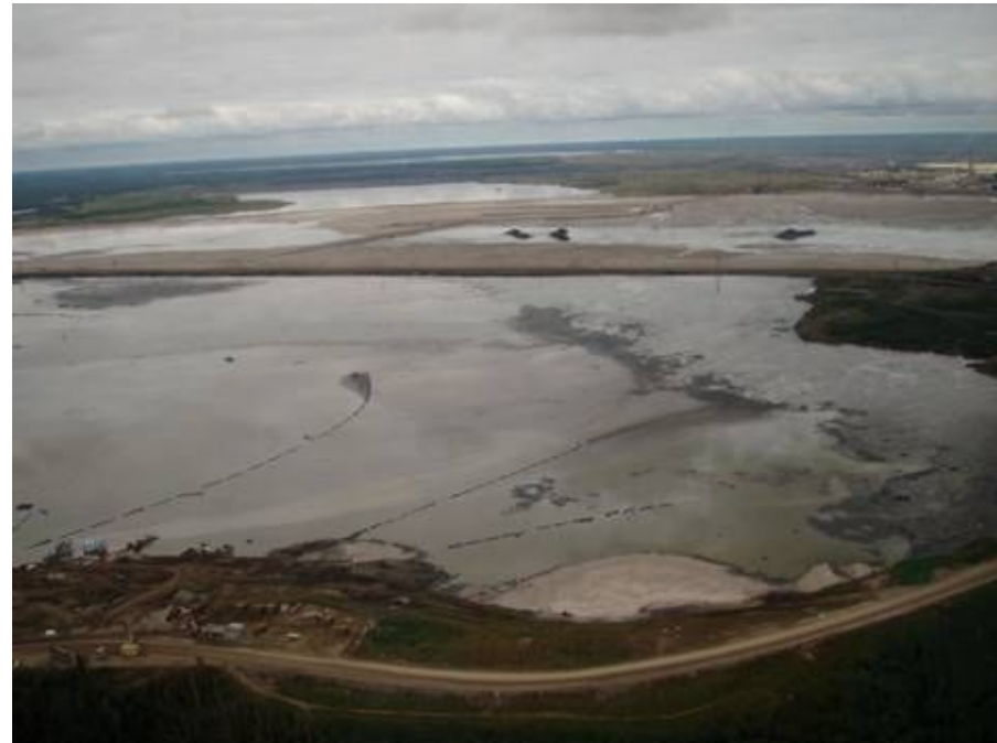
Ponds contain water, residual bitumen and some sand
